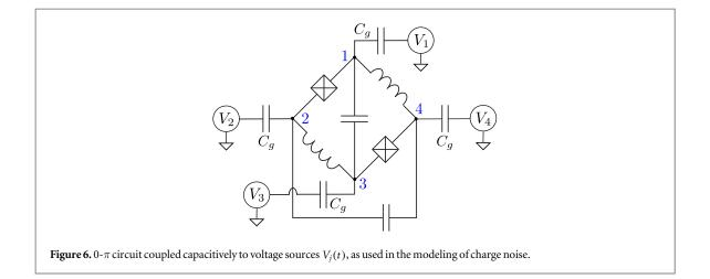
Following [3, 25, 29], we may consider dephasing due to classical noise entering the circuit Hamiltonian in the form of an external parameter  $\lambda(t) = \lambda_0 + \delta\lambda(t)$ . Here,  $\delta\lambda(t)$  is a noise signal assumed to arise from a stationary, Gaussian process with zero mean,  $\langle \delta\lambda(t) \rangle = 0$ , and spectral density
