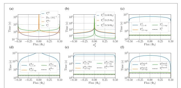
**Figure 7.** Calculated coherence times for parameter set 1. (a) Pure dephasing times due to 1/f flux noise  $T_{\varphi}^{\text{dext}}$  (orange curve), 1/f critical current noise  $T_{\varphi}^{\text{fl}}$  (green curve) as well as shot noise  $T_{\varphi}^{\text{SN}}$  (blue curve), with its approximation  $\kappa_{\zeta}[4\chi_{01}^2 n_{\text{th}}(\Omega_{\zeta})(n_{\text{th}}(\Omega_{\zeta}) + 1)]^{-1}$  from
