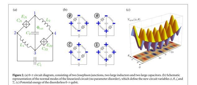
Conceptually, the  $0-\pi$  circuit exhibits a rudimentary form of topological protection that combines exponential suppression of noise-induced transitions (dissipation) with exponential suppression of dephasing, see figure 1. The former is achieved by engineering qubit states with disjoint support, the latter by rendering qubit states (nearly) degenerate and exponentially suppressing the sensitivity of the corresponding energies to low-frequency environmental noise.
