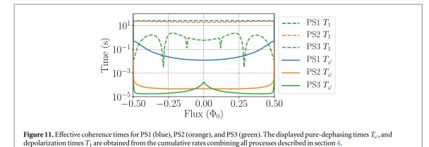
near such dips, we expect the dispersive approximation to break down. There, the qubit is no loner protected by its detuning from the  $\zeta$ -mode, which results in rates that increase the effective depolarization [51].
