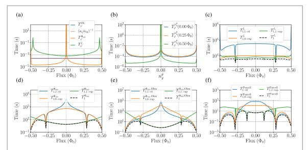
**Figure 9.** Calculated coherence times for parameter set 3. (a) Pure dephasing times due to 1/f flux noise  $T_{\varphi}^{\Phi_{\text{ext}}}$  (orange curve), 1/f critical current noise  $T_{\varphi}^{I_c}$  (green curve) as well as shot noise  $T_{\varphi}^{\text{SN}}$  (blue curve), with its approximation  $1/\kappa_{\zeta} n_{\text{th}}(\Omega_{\zeta})$  (dashed red line),
