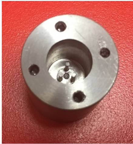
Figure 4.2: Left. Niobium 3 post cavity used to test how to achieve high quality factors with a YIG sphere in the cavity that is biased with a magnetic field. In the center of the 3 posts is a small indentation in which the YIG will rest. Right. Temperature dependence of the quality factor of the niobium cavity without and YIG sphere or field. This set the limit on the maximum quality factors we can obtain in these cavities of \sim 1 million (unless further surface treatment techniques are implemented).
