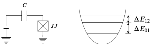
Fig. 17. Left: an LC circuit. In SC LC circuits, normal current becomes SC current. Right: the energy potential of a harmonic oscillator. In QHOs like the SC LC circuits, the system energy becomes equally spaced discrete values. The plotted two levels are the ground state and the first excited state.
